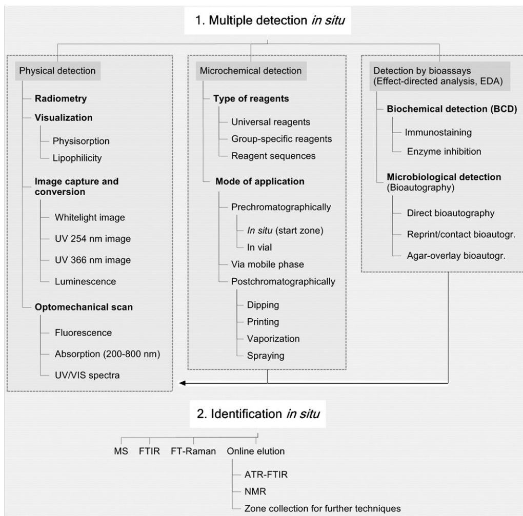
Fig. 5. Potential for hyphenations: multiple detection and identification options for many samples in parallel with a single chromatographic HPTLC separation.
